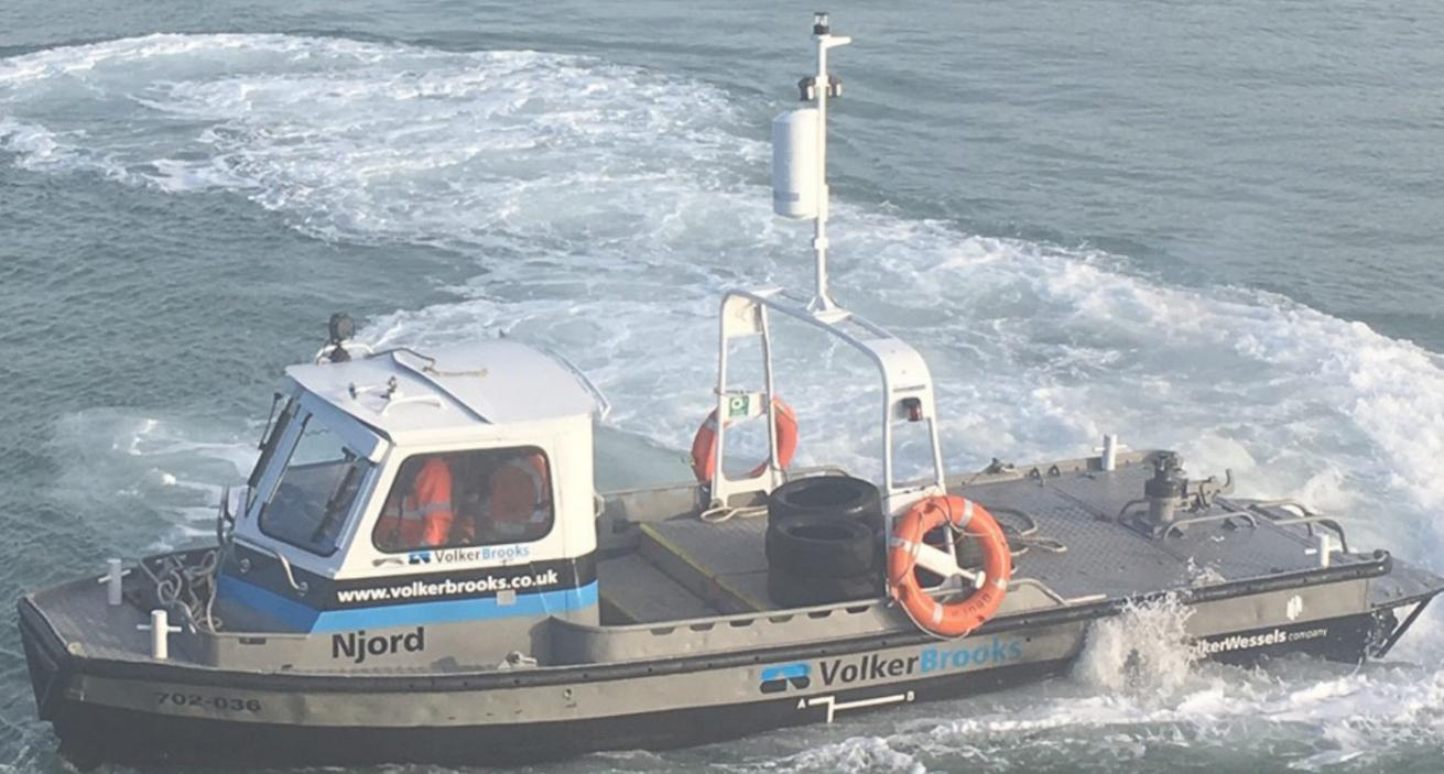
This vessel has been assessed as a Category 6 vessel, as defined within the MGN280 (with a one-mile restriction and only to be operated in favourable weather). Usually, it would be daylight only operations on this provision, however, the vessel may be used as above, but with a Category 3R restricted provision, if all safety equipment is on board to support this operation. Suitable risk assessments and method statements also need to have been completed.
